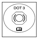
The brake master cylinder reservoir is filled with DOT 3 brake fluid. See *Engine Compartment Overview on page 6-16* for the location of the reservoir.
